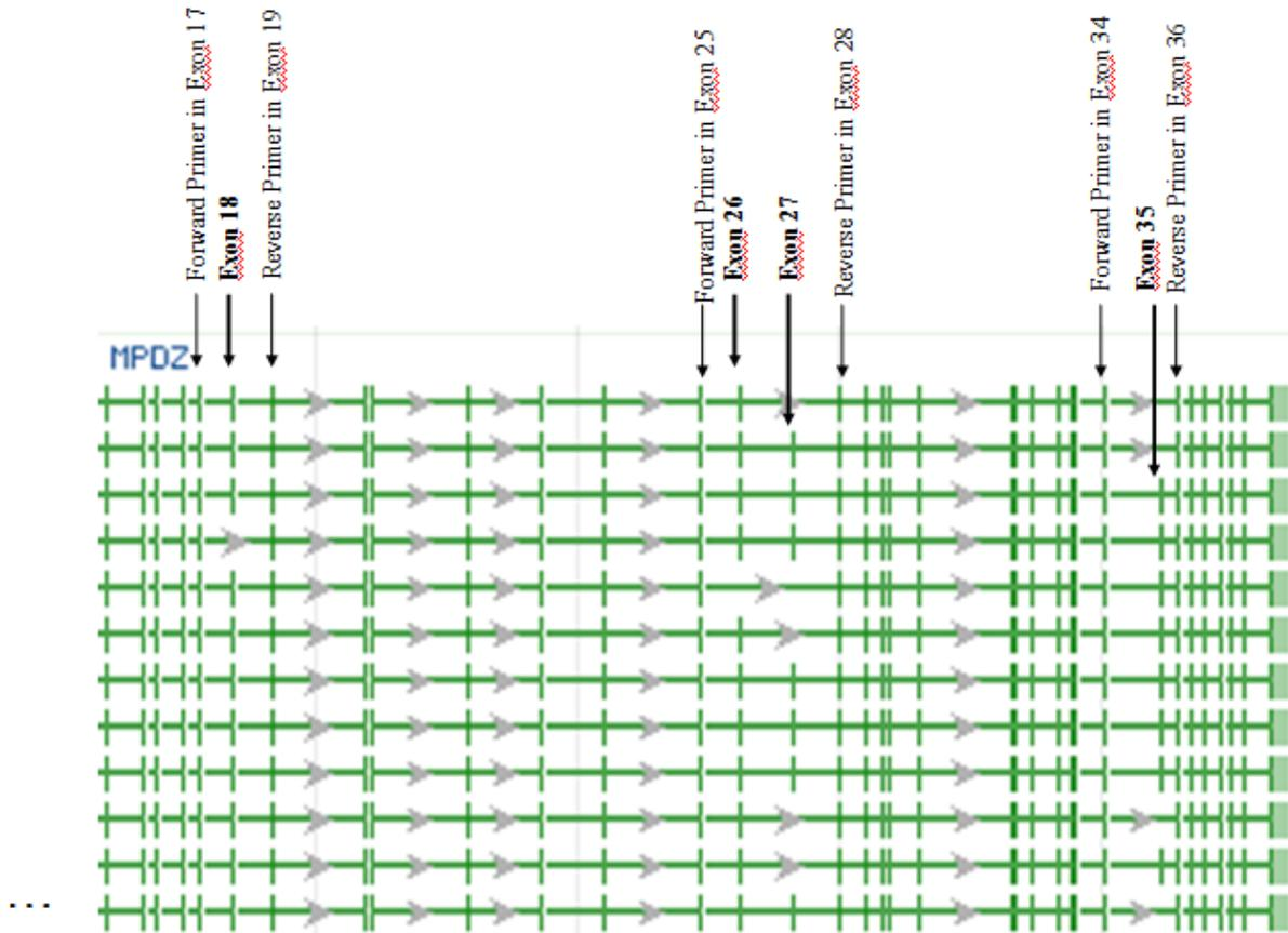
Figure 2: The C-terminal end of MUPP1's gene table from the NCBI website. Each horizontal line represents one variation of MUPP1's transcript. The vertical lines represent exons and the horizontal lines in between them symbolize introns. Primers were designed to amplify the exons missing in some transcripts.
